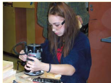
Jolene Nowak uses a router to produce a keyhole slot.
